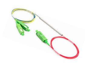
Agiltron's double-clad 2x2 fiber coupler combines a double-clad fiber (single mode core surrounded by a multimode inner cladding) with a large core multimode fiber. Light in the single mode core of the double-clad fiber (DCF) is guided through the coupler with little loss (≤0.5 dB). Light in the multimode inner cladding of the DCF is transferred to the output multimode fiber with ≥60% transmission.
